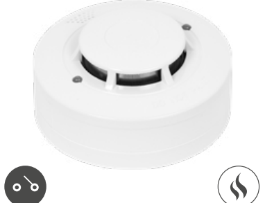
Optical Smoke Detector FDR26 Covered space: 40m², max. height 7m
