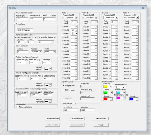
With clicking on the button "Load RK-CHM-D" the configuration values from the flash memory of sensor are read.
