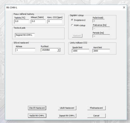
With clicking on the button "Load RK-CHM-L" the configuration values from the flash memory of sensor are read.
